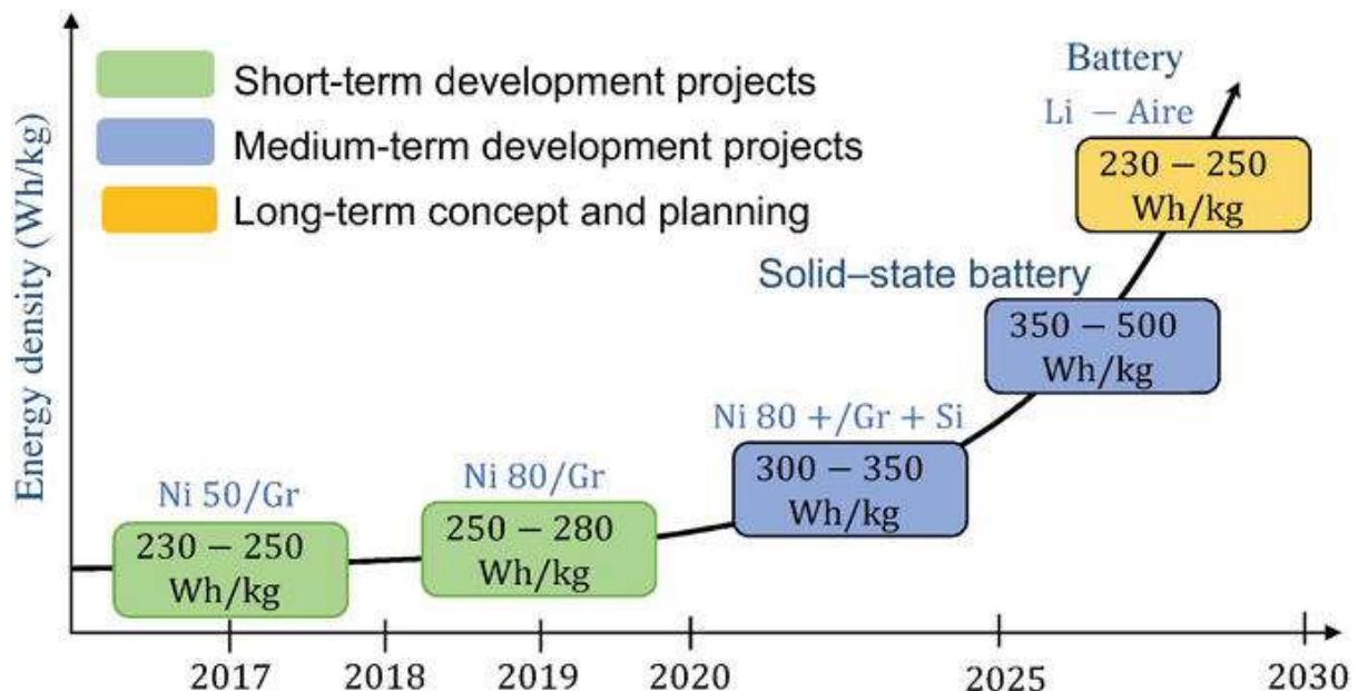
Figure 5. Increased energy density of batteries.
